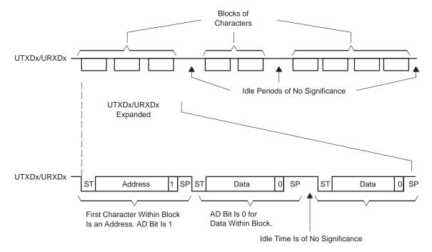
For address transmission in address-bit multiprocessor mode, the address bit of a character can be controlled by writing to the TXWAKE bit. The value of the TXWAKE bit is loaded into the address bit of the character transferred from UxTXBUF to the transmit shift register, automatically clearing the TXWAKE bit. TXWAKE must not be cleared by software. It is cleared by USART hardware after it is transferred to WUT or by setting SWRST.
